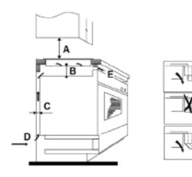
**NOTICE** // The safety distance between the hotplate and the cupboard above the hotplate should be at least 760mm.
